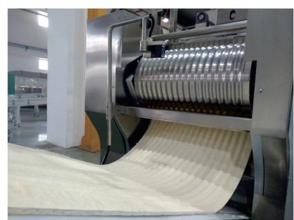
Using the large and medium sized corrugated roll, This dough is malleable and the noodles taste good.
