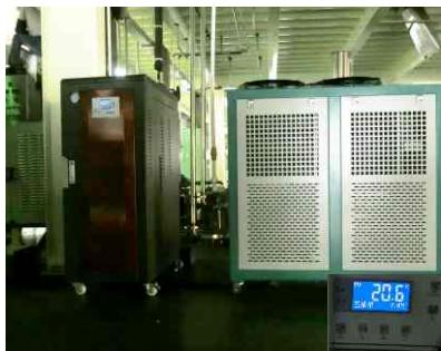
Extruding temperature control system: heating medium adopts steam or electromagnetism; use water chiller for cooling. Heating and cooling are quick and stable; First extrude and scend extrude can be switched freely.
