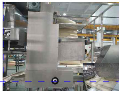
Adopt lateral folding machine, The dough is extended in many rolled directions that makes the noodles taste good.
